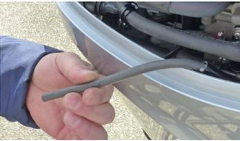
3. Release the drain tube from the projection of the intake manifold and bring the end of the drain tube out from beneath the cover.
