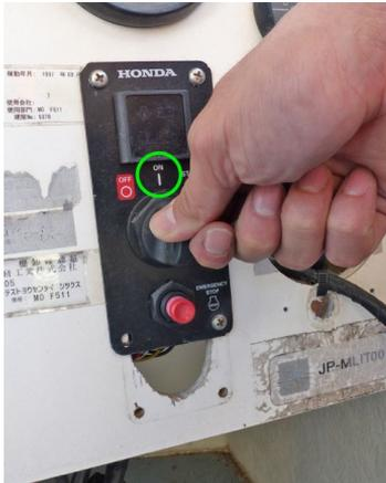
10. Turn the engine switch key to the ON position.
