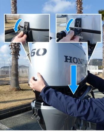
14. Leave the ACG cover off and install the engine cover. Lock the engine cover fixing levers.
