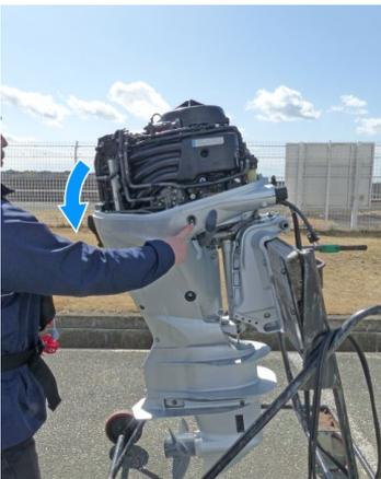
8. Tilt the outboard motor down.
