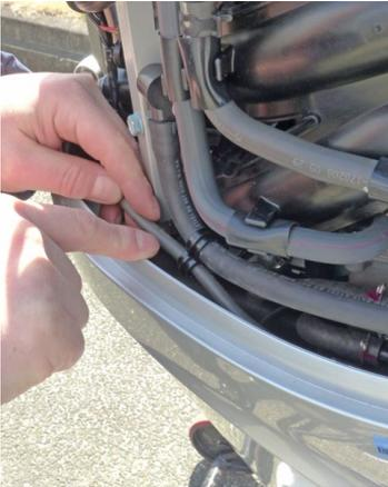
7. Secure the drain tube to the projection of the intake manifold.
