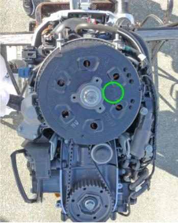
6. Set the ACG rotor so the cutouts are on the right and left sides of the ACG rotor as shown.
