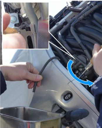
5. Drain the petrol into the drain pan as it flows out of the drain tube.
