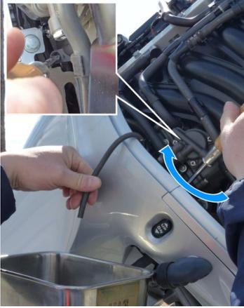
6. After draining, tighten the drain screw.
