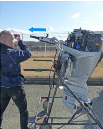
17. Pull the emergency starter rope several times to lubricate the inside of the cylinder. Then remove the emergency starter rope.
