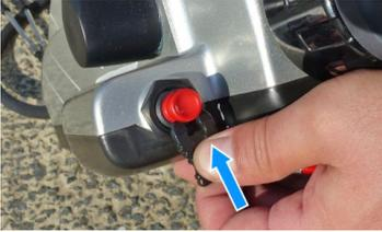
9. Insert the emergency clip into the emergency stop switch. Attach the other end of the emergency stop switch lanyard securely to the operator.
