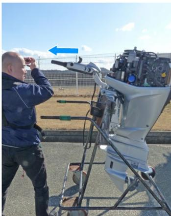
11. Pull the starter rope lightly until resistance is felt, then pull firmly.
