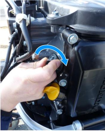
18. Carefully install the spark plugs by hand to avoid cross-threading. Tighten  $1/8$ – $1/4$  turn after the spark plug seats. Install the ACG cover.
